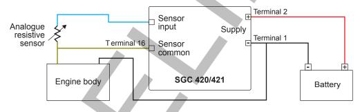
\*SCP connections for Analogue input 2 used as Fuel level sensor with the reference configured as Battery Negative
